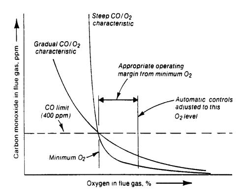
**Figure 2** Oxygen/Smoke Characteristic Curve
