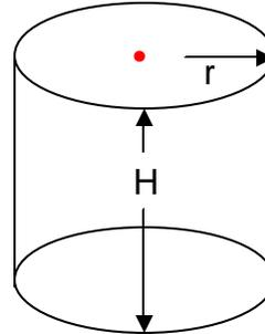
$$\text{Volume of the cylinder} = \pi r^2 H = 3.14 \times 36^2 \times 12 = 48,858 \text{ in}^3$$
