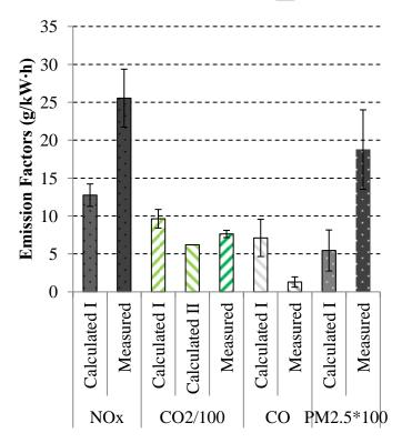
Calculated I: EPA method; Calculated II: CARB method
