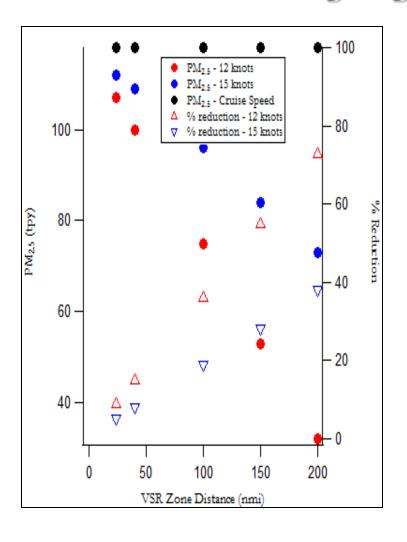
TPE<sub>PM2.5</sub> reduction almost doubled on reducing large vessel speed from 15 knots (5-38%) to 12 knots (9-73%)
