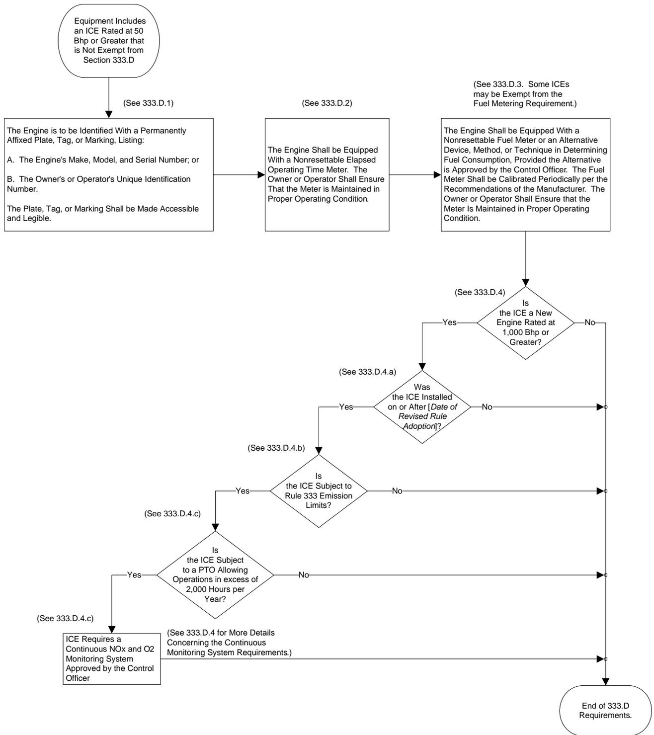
Figure 2. Rule 333 Provisions on Engine Identification, Meters, and Continuous Monitoring Systems.<sup>1</sup>
