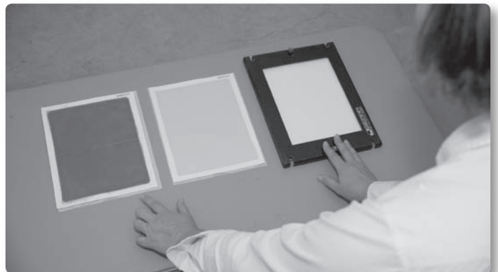
The dark colored particulate filter from the Las Flores Canyon monitoring station, located in a canyon area near El Capitan, shows the high level of particles in the surrounding air from midnight October 21 to midnight of October 22. The other two filters are a filter from the same monitoring station exposed from midnight October 3 to midnight October 4, and an unexposed filter.
