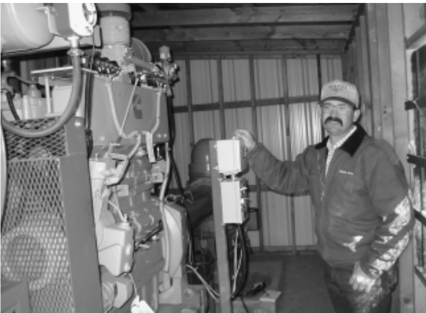
Cliff Dugger of Teixeira Farms demonstrates the new propane-powered water pump engine, equipped with a catalytic converter, purchased with funding from APCD.
