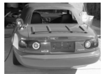
The vehicle can travel up to 50 miles before recharging.
