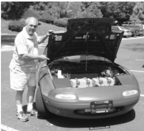
Engineer Bill Theeringer shows off his electric Miata, which he converted in his garage from a gasoline-powered Miata, using off the shelf equipment.
