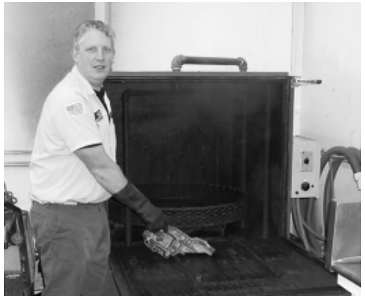
Dan Giers demonstrates a water-based auto parts washer currently in use at Malmcke Motors in Goleta.
