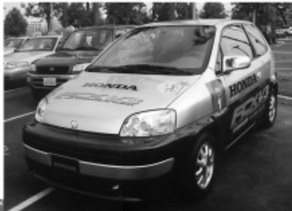
Below: The Honda FCX V3, powered by a fuel cell combined with an ultracapacitor, which contributes to acceleration performance.
