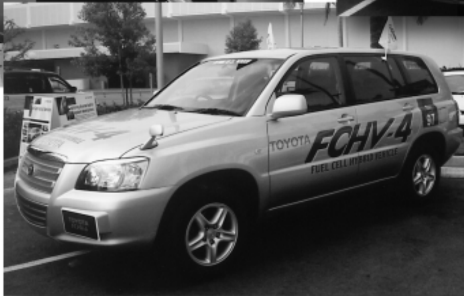
Left: APCD Director Doug Allard takes a ride in the Toyota FCHV-4, a prototype fuel cell hybrid vehicle demonstrated at the recent Clean Air Technologies 2001 conference. The FCHV-4, expected to be available in limited quantities in 2003, is powered by a 90kW fuel cell stack, and a secondary nickel-metal hydride battery that provides additional power.
